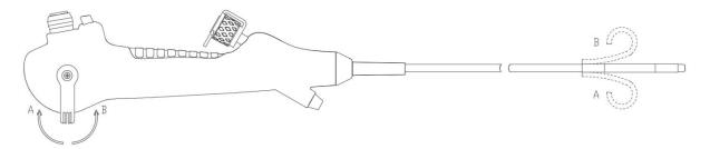
3.4.3 Slowly slide the bending control lever to the neutral position and confirm that the bendable portion can be smoothly restored to a nearly straight line
