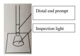
3.3.3 Point the distal tip of the endoscope at the object to be measured and move it between 3-50 mm. Verify on the monitor that the image quality and brightness of the object to be measured are basically stable.
