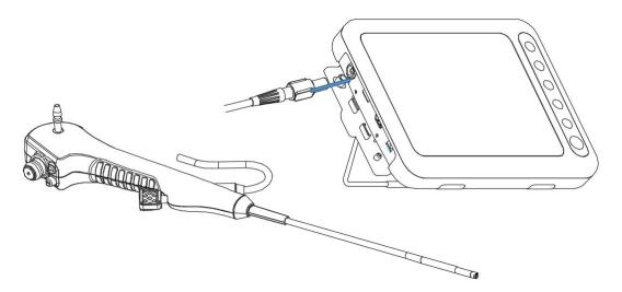
3.3.2 Confirm that there is a beam of light emitted from the end of the endoscope (dual LED)
